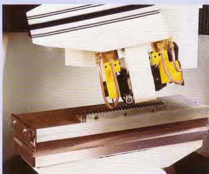
Grinding flat broaches requires high flexibility from the grinding head with the D axis. It is visible here for grinding – from left to right – the flute, the clearance face and the chipbreaker
