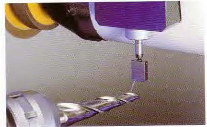
A measuring probe which is rigidly mounted onto the grinding head performs the automatic tool positioning – shorter grinding cycle
