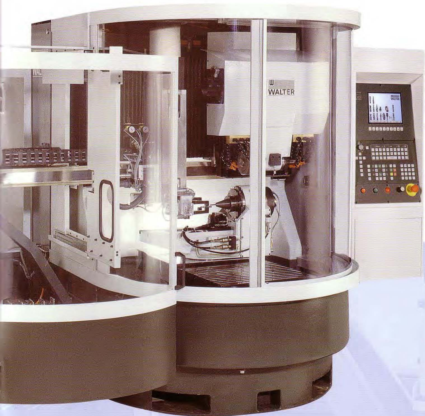
Helitronic Power Production with production loader for automatic production grinding in several shifts. The grinding machine is programmed for the next pallet whilst the grinding of the tools on the pallet is completed. The grinding cycle starts immediately after the change of pallet.
