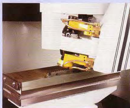
Grinding flat broaches requires high flexibility from the grinding head with the D axis. It is visible here for grinding – from left to right – the flute, the clearance face and the chipbreaker
